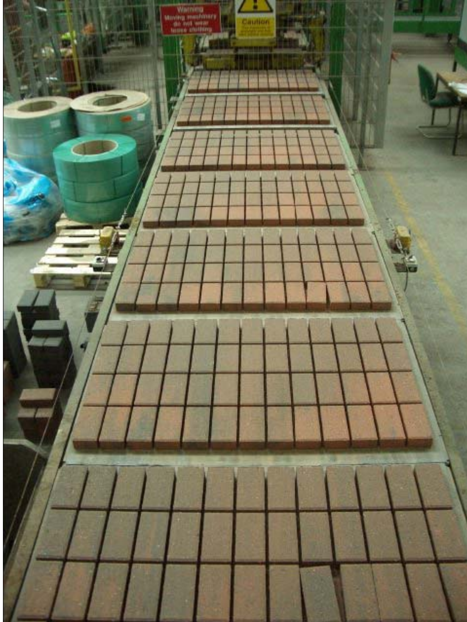
Freshly cured products leaving the chamber
