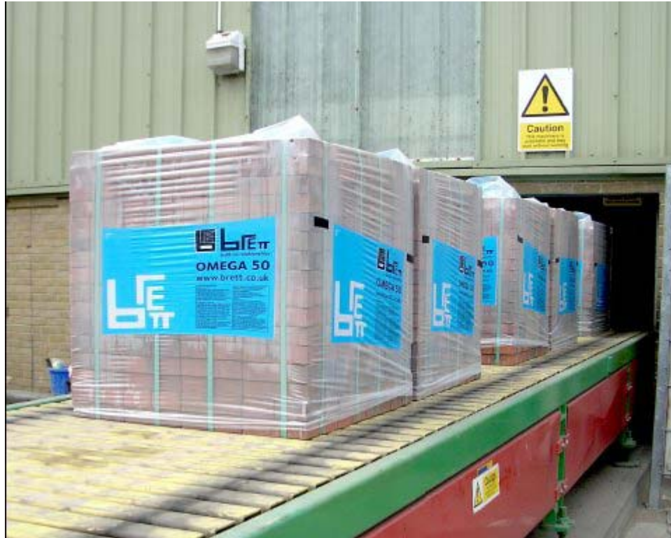
Slat conveyor carrying products into the yard
