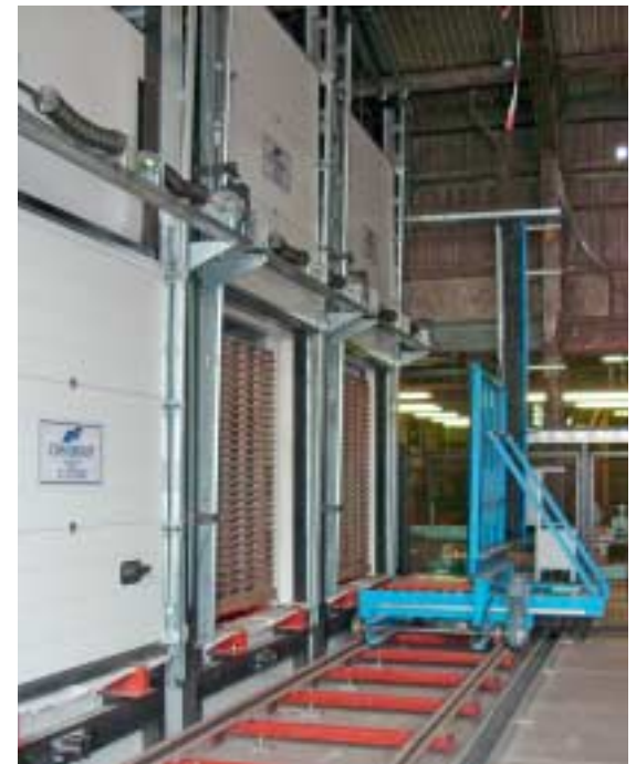
Fig. 4 View showing the entry end transfer car and track with tiles exiting the initial conditioning lane.
