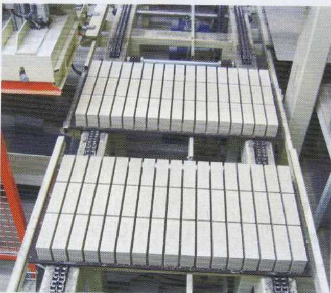
Transport system on the dry side
