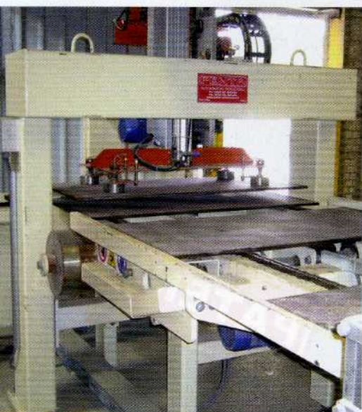
Positioning of the steel pallets with magnets for the block machine
